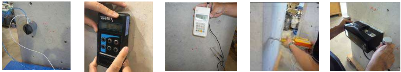
(a) Air permeability test (b) Water content test (Surface) (c) Water content test (Inside) (d) Rebound number test (e) Ultrasonic test
