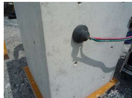
Fig.5 Air permeability test
