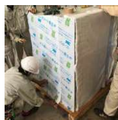
(c) Sealed curing
