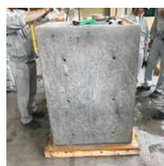
(a) Atmospheric curing
