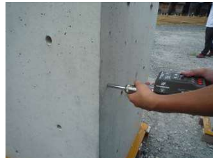
Fig. 6 Rebound number test
