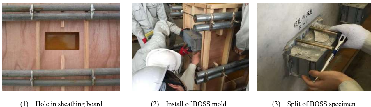
Fig. 1 Method for make BOSS specimen
