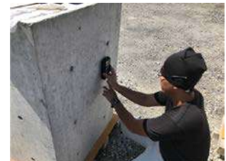
Fig. 4 Water content test (Surface)
