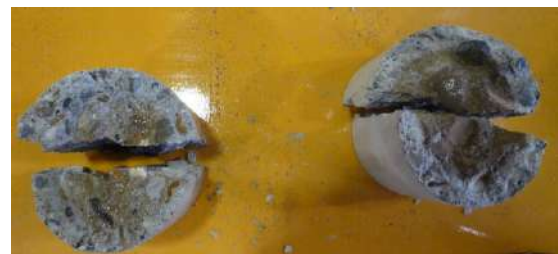
Discolored boundary by chloride ions
