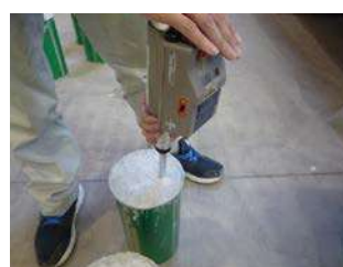
Fig.5 Rebound hammer test
