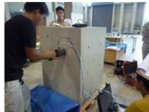
Fig. 3 Air permeability test
