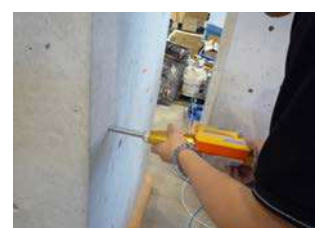
Fig. 6 Rebound number test
