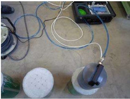
Fig.7 Air permeability test
