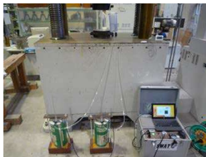
Fig.8 Water absorption test
