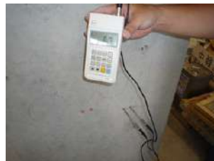
Fig. 5 Water content test (Inside)
