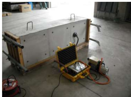
Fig.3 Measurement of air permeability
