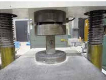
Fig.4 Compressive strength test
