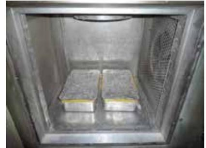
Fig.3 Hot-water curing for 48 hours
