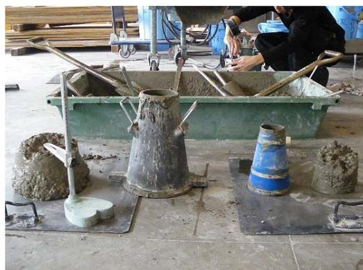
Fig. 4 Slump test and mini-slump test
