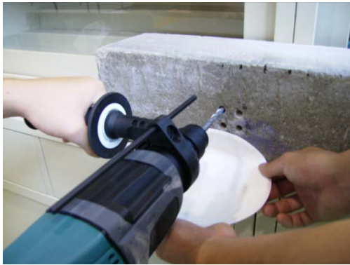
Fig.1 Drill concrete specimen
