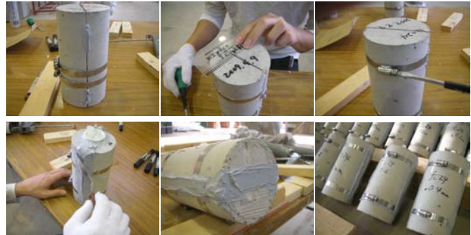
Fig. 2 Control of crack width and preparation of injecting epoxy resins
