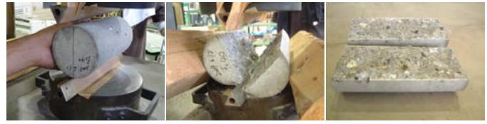
Fig. 1 Method of splitting specimens
