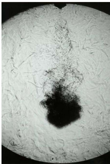
Fig.10 Visualized soot in a diesel flame (combustion chamber diameter: 196 mm)
