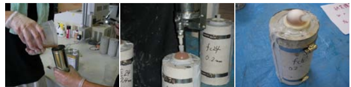
Fig. 3 Injection of epoxy resins into concrete cracks
