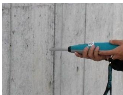
Fig. 2 Rebound speed ratio test
