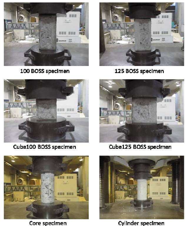
Fig.7 Compressive strength test
