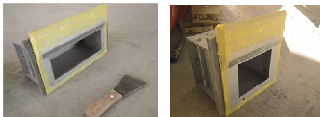
Fig.1 Prism BOSS mold and Cube BOSS mold
