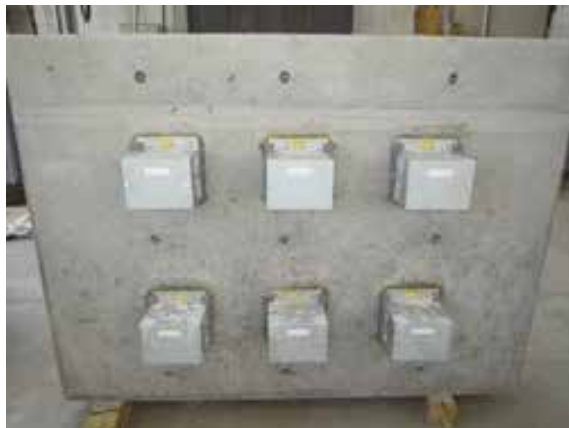
Fig.5 Sealed curing of BOSS specimen
