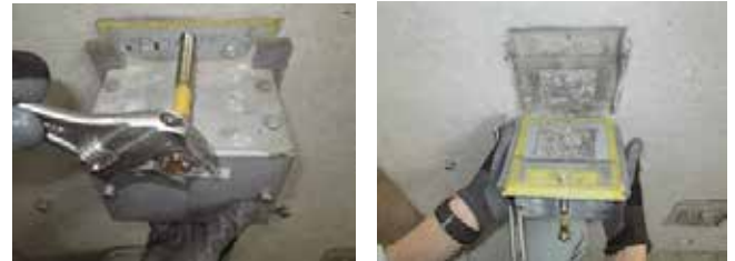
Fig.6 Break off BOSS specimen by splitting
