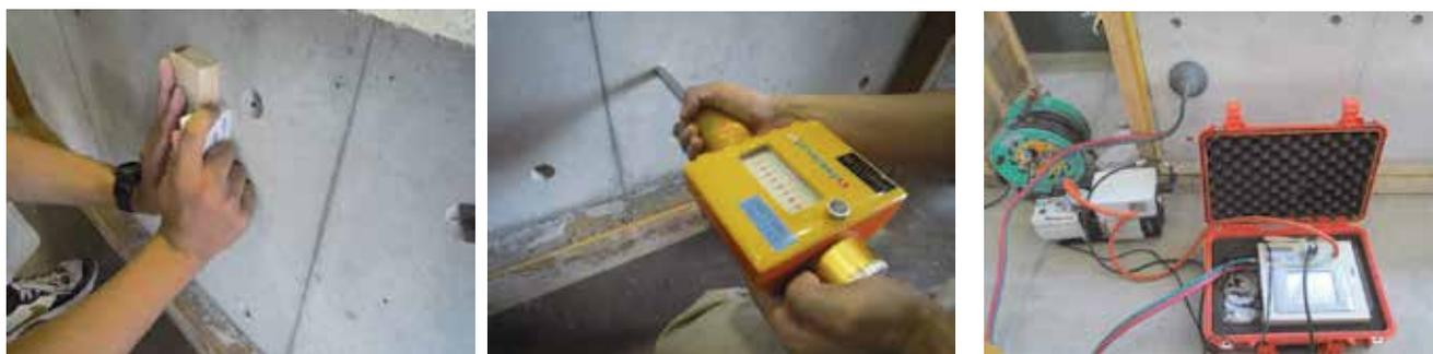
Fig.4 Measurement of concrete surface hardness
