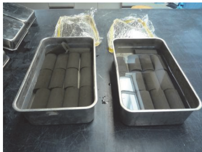
Fig.2 Preparation for hot-water curing
