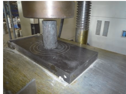
Fig.6 Compressive test after fire resistance test
