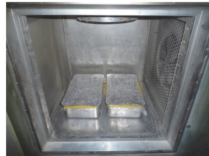
Fig.3 Hot-water curing for 48 hours
