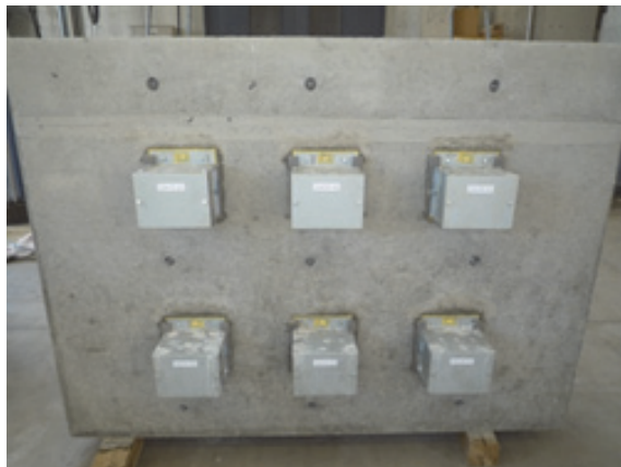
Fig.5 Sealed curing of BOSS specimen
