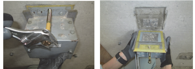
Fig.6 Break off BOSS specimen by splitting
