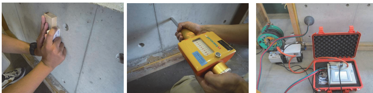
Fig.4 Measurement of concrete surface hardness
