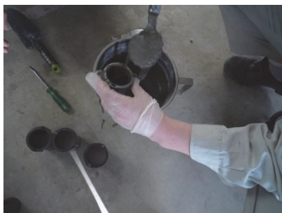
Fig.1 Placement of concrete
