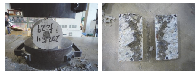
Fig.7 Tensile strength test
