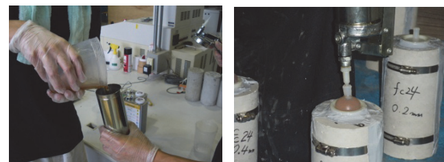
Fig.5 Injection of epoxy resin into concrete cracks
