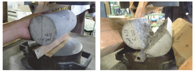
Fig.1 Method of splitting specimens
