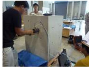
Fig. 3 Air permeability test
