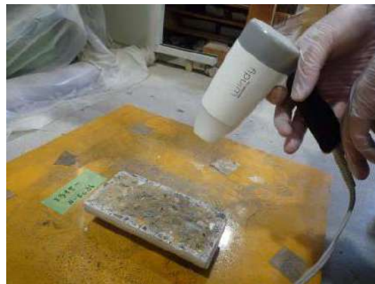
Photo. 8 Dry specimen with hair drier for a minute (BB Fc36)
