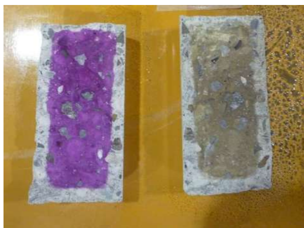
Spray \text{C}_{20}\text{H}_{14}\text{O}_4 solution Spray \text{AgNO}_3 solution
