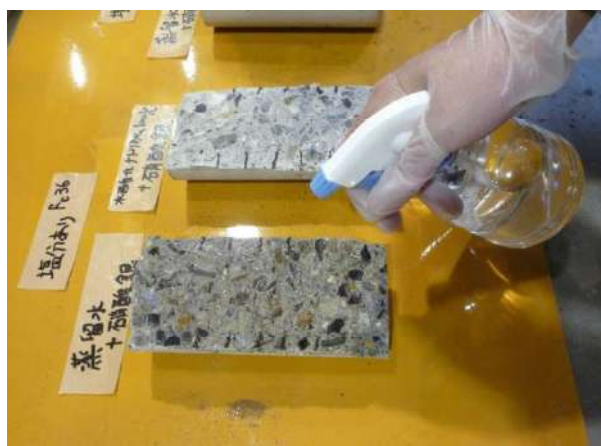
Photo. 3 Spray distilled water
