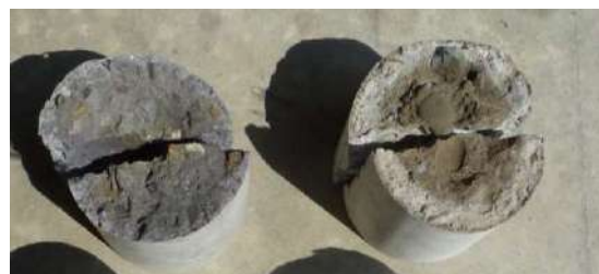
Discolored boundary by chloride ions
