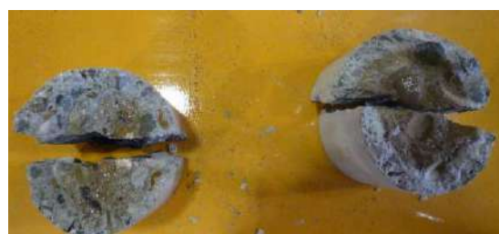
Discolored boundary by chloride ions
