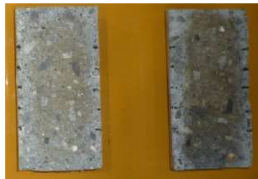
Spray \text{AgNO}_3 solution
