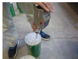
Fig.5 Rebound hammer test
