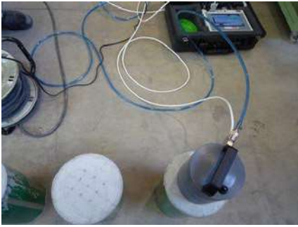
Fig.7 Air permeability test
