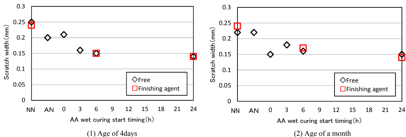
Fig.10 Effects of curing methods on scratch width
