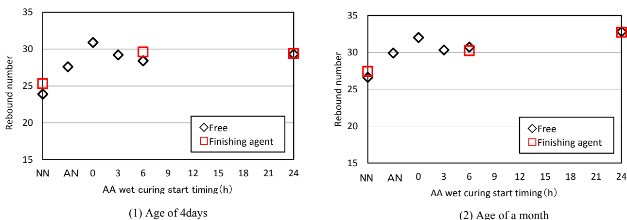
Fig.11 Effects of curing methods on rebound number
