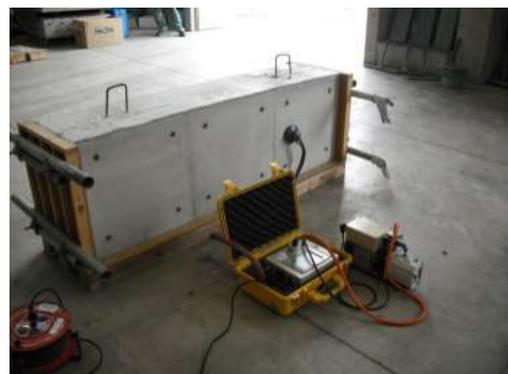
Fig.3 Measurement of air permeability
