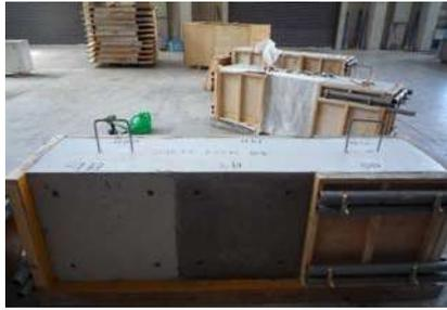
Fig.1 Preparation of wall specimen
