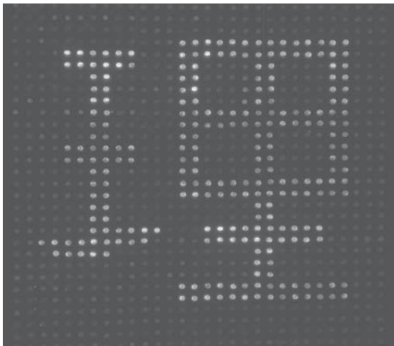
Fig.3 Photograph of the display part for the possibility of tiled-vision. 9 display units arrange to 3 × 3. 30 × 30 pixels display is constituted.
