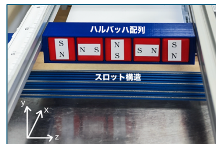
図3 吸引力測定実験 Fig.3. Attraction force measurement experiment
